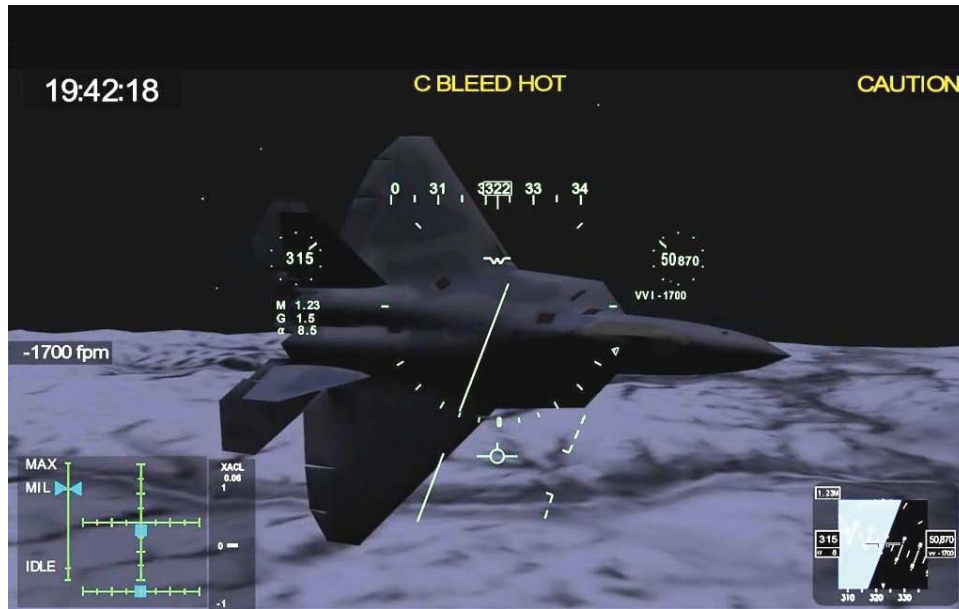
Figure 2 19:42:18 -- MA parameters at assertion of C BLEED HOT caution ICAW. (Tab EE) See Tab Z-10 for a diagram explaining the symbology in the Figures.
