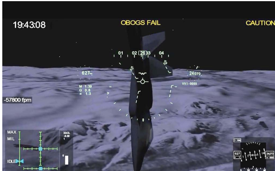
Figure 7 19:43:08 – MA parameters when stick and pedal inputs cease after the 240 degree roll. (Tab EE)
